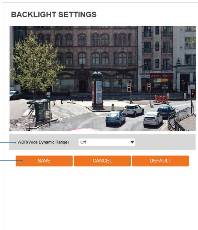
**This feature is used when lighting conditions may cause detail loss in the camera's view due to high contrast.**
