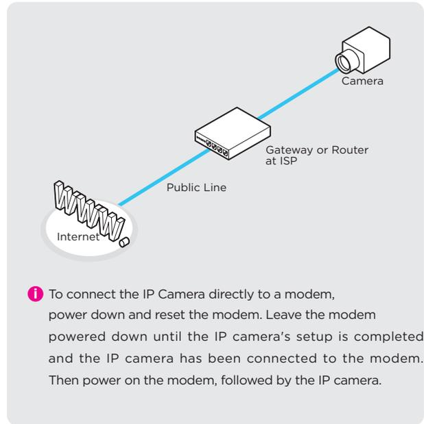
**i** To connect the IP Camera directly to a modem, power down and reset the modem. Leave the modem powered down until the IP camera's setup is completed and the IP camera has been connected to the modem. Then power on the modem, followed by the IP camera.
