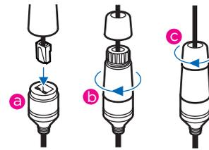
NOTE: To ensure moisture seal, make sure the o-ring is in place between (a) and (b). In extreme environments use of an outdoor rated sealer is recommended.
