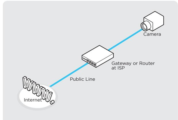
**i** To connect the IP Camera directly to a modem, power down and reset the modem. Leave the modem powered down until the IP camera's setup is completed and the IP camera has been connected to the modem. Then power on the modem, followed by the IP camera.
